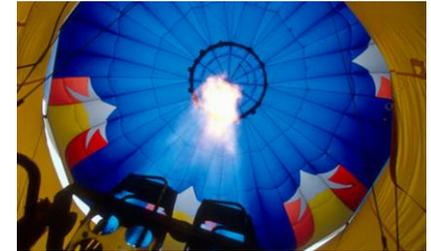
A hot air balloon must be filled with air and the air must be heated for the balloon to be able to lift off the ground. The air has to be kept warm of the balloon will fall.
