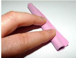
Rolling paper to create a paper roll can make it stronger. The longer the pole, the less strength it provides.
